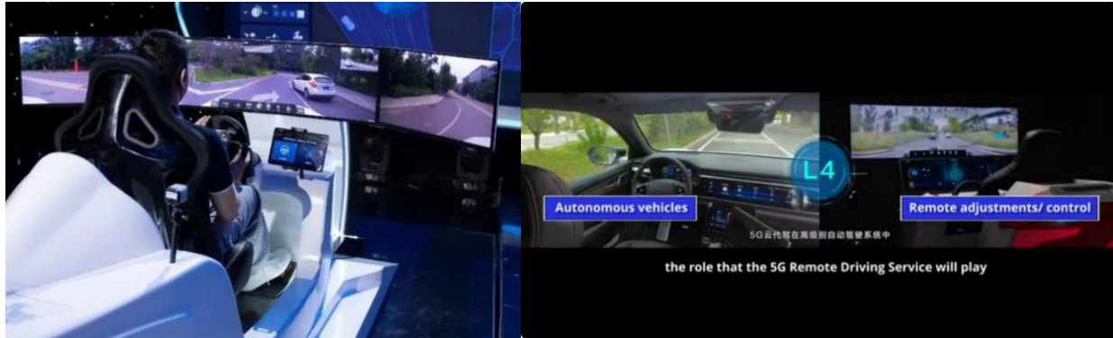
Figure 7. (Left) Baidu's remote operation station; (Right) Baidu's 5G Remote Driving with the autonomous system and the remote operator (Apollo Auto, 2020).
