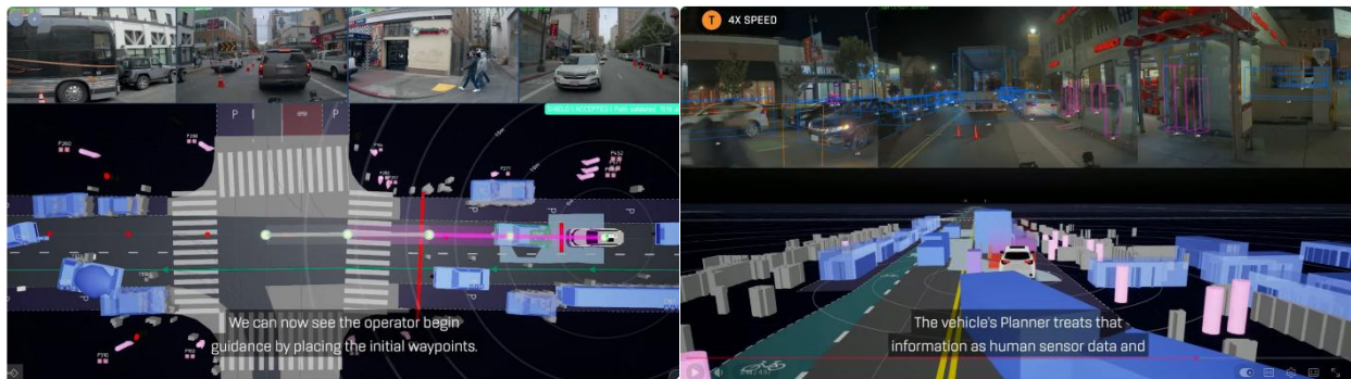
Figure 6. (Left) Zoox's remote operator suggests a path by placing waypoints; (Right) Zoox's remote operator labels a parked truck in front of the robotaxi as an obstacle (Zoox, 2024a).
